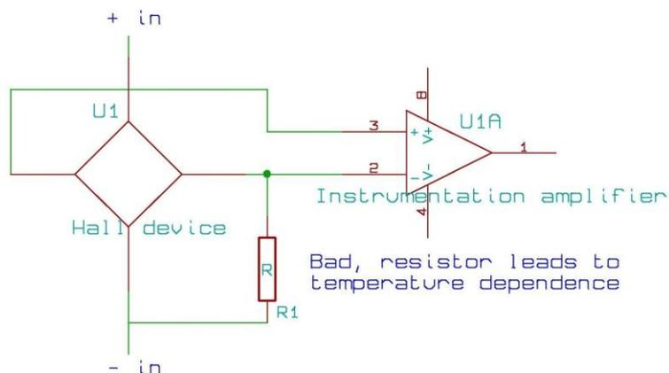
The example above leads to a temperature drift of the offset voltage. Meaning that the offset voltage is not constant but changes with temperature and is difficult to compensate.
