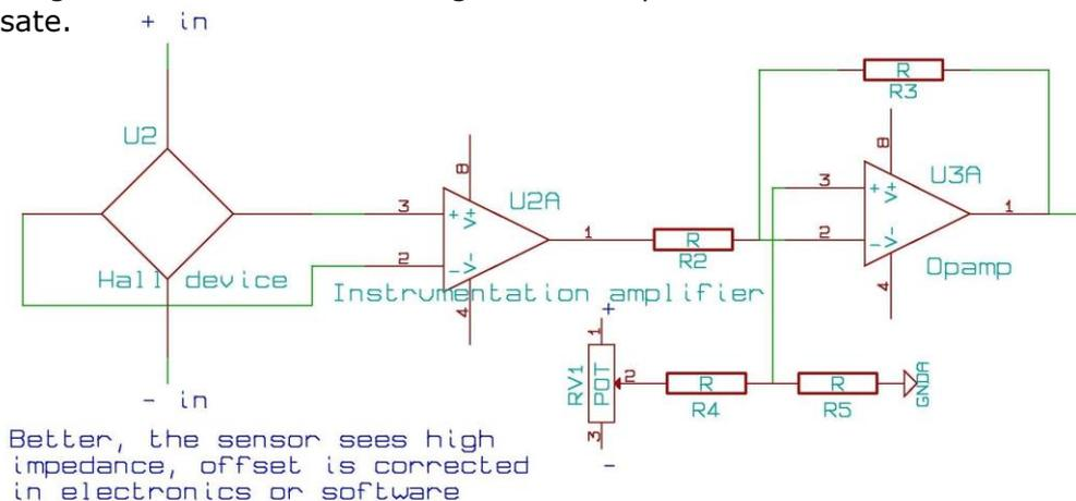
This is just an example of an offset voltage correction that gives good results. There are many other ways to compensate for offset voltages. As the electronics already has a current source, it is good practice to use the reference used for that current also as reference for compensation of offset voltages. This will cancel out part of the temperature drift of your electronics.
